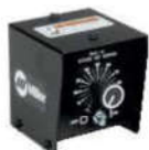
RFCS-14 HD Foot Control 194744 Maximum flexibility is accomplished with a reconfigurable cord that can exit the front, back or either side of the pedal. Foot pedal provides remote current and contactor control. Includes 20-foot (6 m) cord and 14-pin plug.
