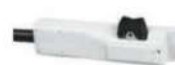
RMLS-14 Switch 129337 Momentary- and maintained-contact rocker switch for contactor control. Push forward for maintained contact and backward for momentary contact. Includes 26.5-foot (8 m) cord and 14-pin plug.
