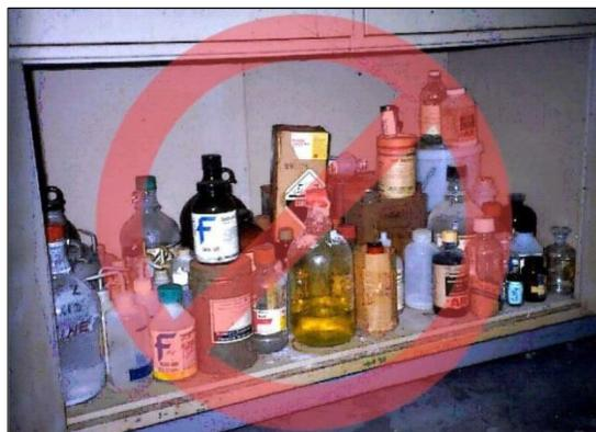
Laboratory shelves should have a raised lip along the outer edge to prevent containers from falling. Hazardous liquids or corrosive chemicals should not be stored on shelves above eye-level and chemicals which are highly toxic or corrosive should be in unbreakable secondary containers.
